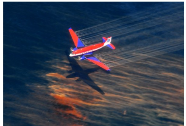
Aerial application of dispersants to an oil slick. Photo courtesy of the
