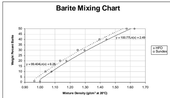
Figure 1. Chart for calculating oil/barite density
