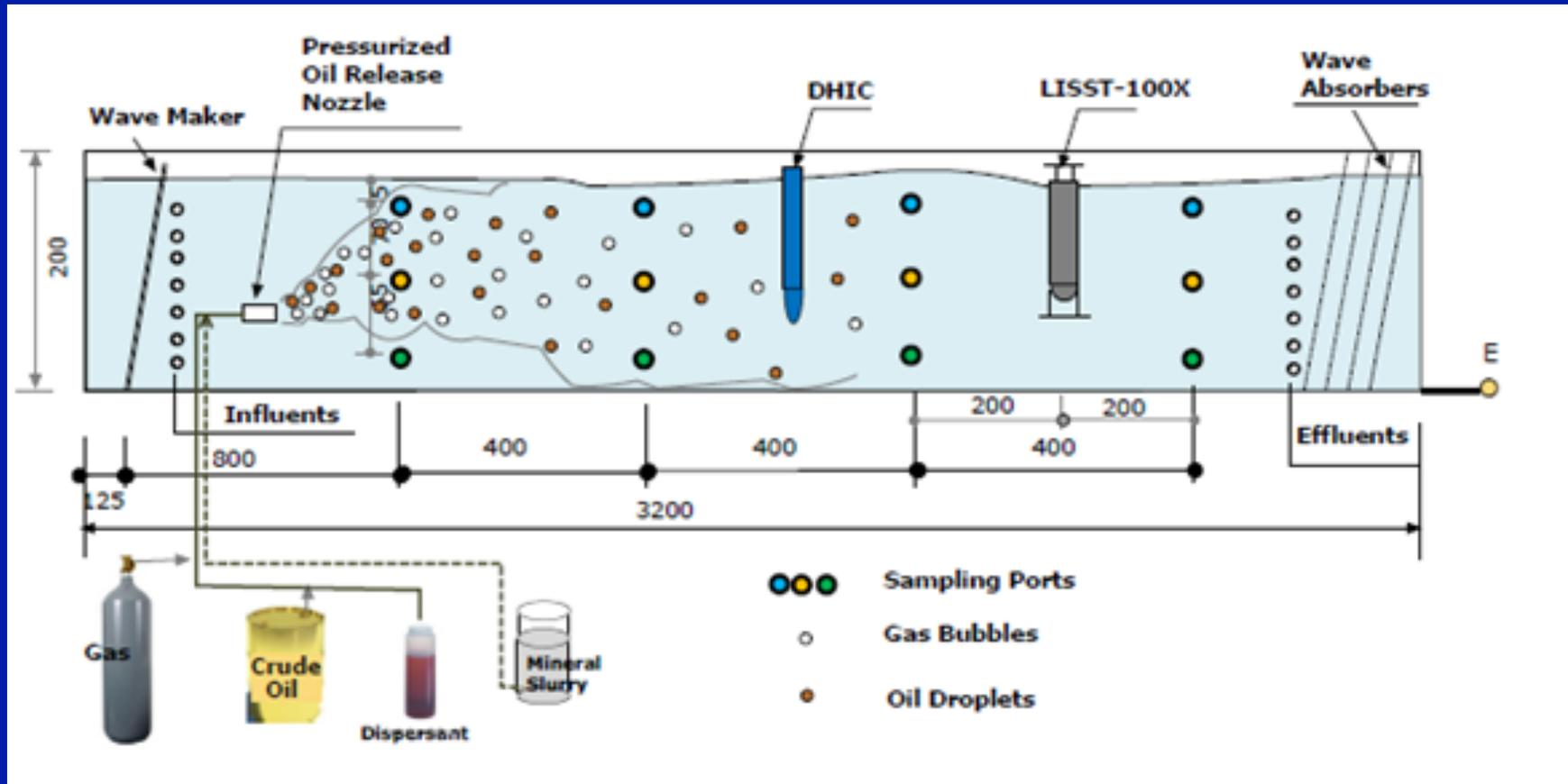
DHIC: Digital Holographic Imagery Camera, to measure particles 20 – 2500  $\mu\text{m}$
