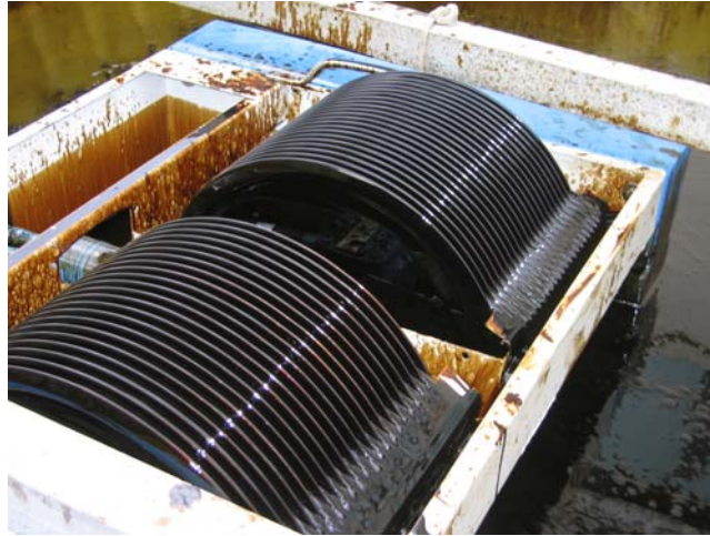
Figure 2. Elastec™ Mini Max® drum skimmer. Standard drums were replaced with grooved drums and a matching scraper.
