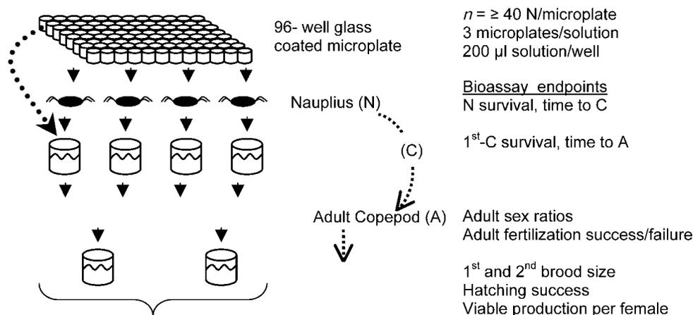
Fig. 1. Experimental setup of the full life-cycle bioassay exposing the copepod *Amphiascus tenuiremis* to National Institute of Standards and Technology (NIST) crude oil water-accommodated fraction (WAF) dilutions and seawater control (0% WAF) under ultraviolet (UV) and fluorescent (non-UV) regimes. A = adult copepod; C = copepodite; N = nauplius.
