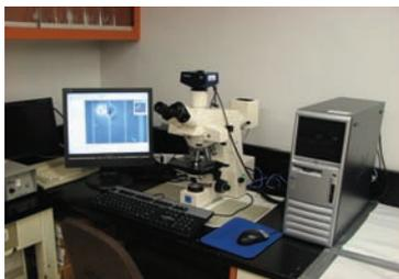
**FIGURE 5** IMAGING SETUP USED TO PICTURE OSAS USING UV EPI-FLUORESCENCE MICROSCOPY AND A HIGH RESOLUTION ZEISS DIGITAL CAMERA CONTROLLED WITH A COMPUTER. THE SETUP IS DESIGNED TO MEASURE DROPLET SIZE OF 0.1  $\mu\text{m}$  AND LARGER.
