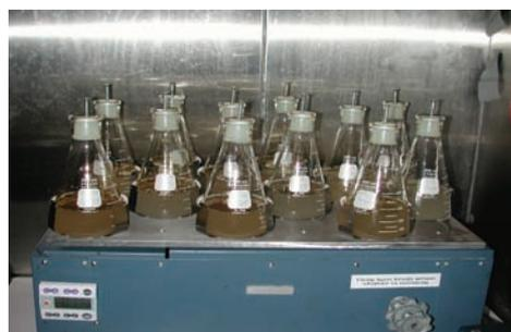
FIGURE 1. REACTION VESSELS SET FOR SHAKING ON THE RECIPROCATING SHAKER
