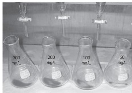
FIGURE 2 REMAINING OIL-SEDIMENT MIXTURE (SINKING OSAS ) AFTER EXTRACTION OF THE FLOATING MATERIALS AND WATER. SAMPLES READY FOR TRANSFER INTO SEPARATORY FUNNELS FOR EXTRACTION. NOTE SEDIMENT CONCENTRATION INCREASES FROM RIGHT TO LEFT.
