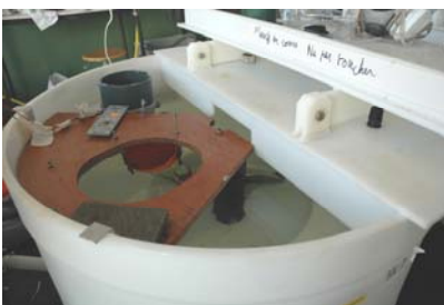
Figure 2 The test tanks with the pumping system designed to keep the oil from resurfacing.
