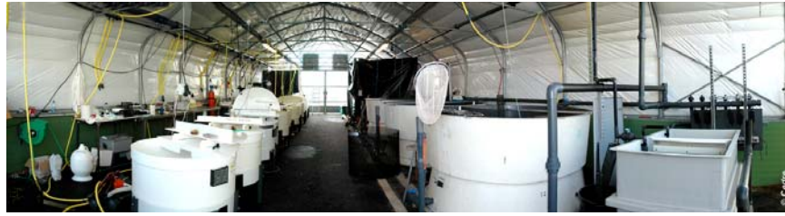
Figure 3 View of the eco-toxicological testing facilities of Cedre: on the left, the 14 tanks used to expose the animals to the pollutant, on the right the stabilization tanks
