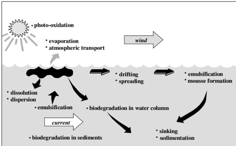
Figure 4-1 Processes Acting on Spilled Oil
