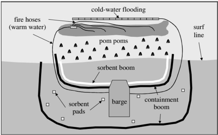
Figure 12-7 Low-Pressure, Warm-Water Washing/Cold-Water Flooding
