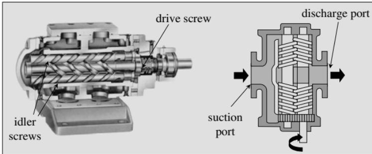
Figure 11-4 Intermeshing Screw Pump
