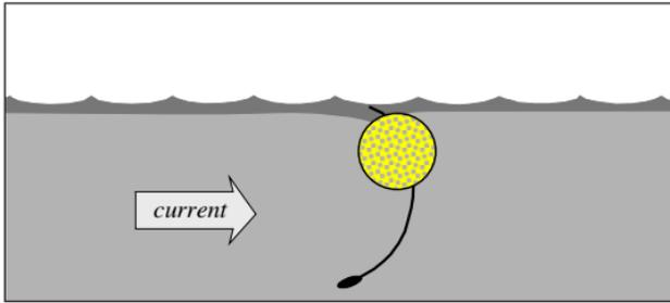
Figure 5-5 Submergence Failure
