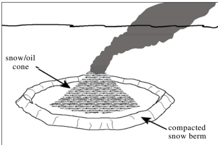
Figure 15-2 Burning Snow Cone (From EPPR 1998)
