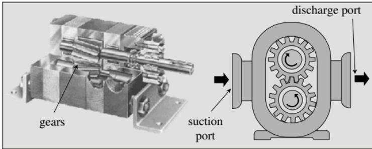
Figure 11-3 Gear Pump
