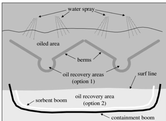
Figure 12-6 Low Pressure Flushing
