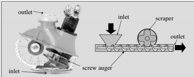
Figure 11-7 Screw/Auger Pump
