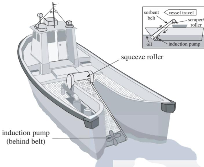
Figure 9-13 Sorbent Lifting Belt
