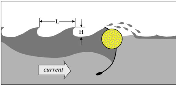
Figure 5-4 Splashover Failure
