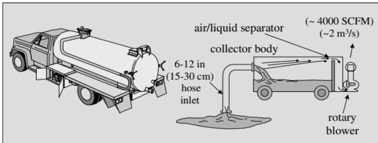
Figure 11-13 Air Conveyor
