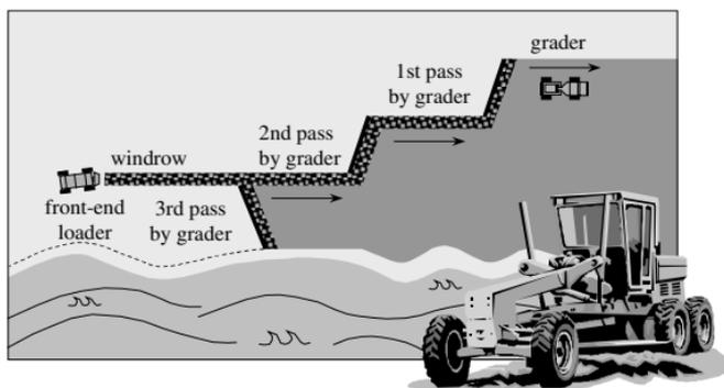
Figure 12-17 Motor Grader/Front-End Loader Combination Treatment Pattern
