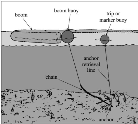
Figure 5-16 Boom Anchoring Assembly
