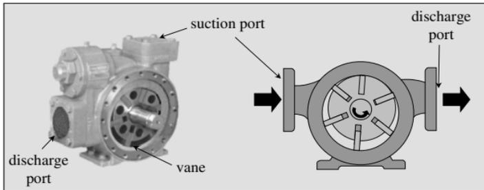
Figure 11-5 Vane Pump
