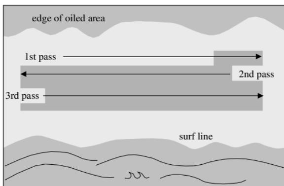
Figure 12-11 Tractor/Ripper Treatment Pattern
