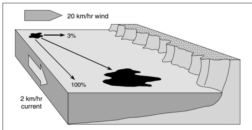
Figure 4-2 Movement of Oil on Water
