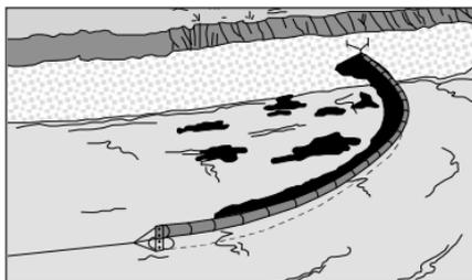
Figure 5-14 Shore-Sealing Boom
