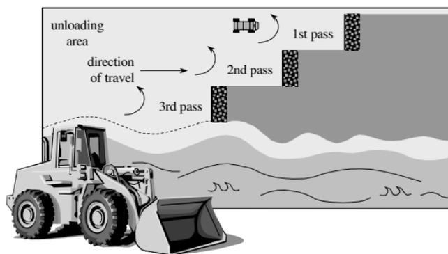
Figure 12-16 Front-End Loader Treatment Pattern
