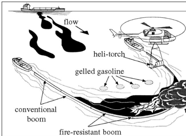
Figure 8-3 Typical In-Situ Burning Operation
