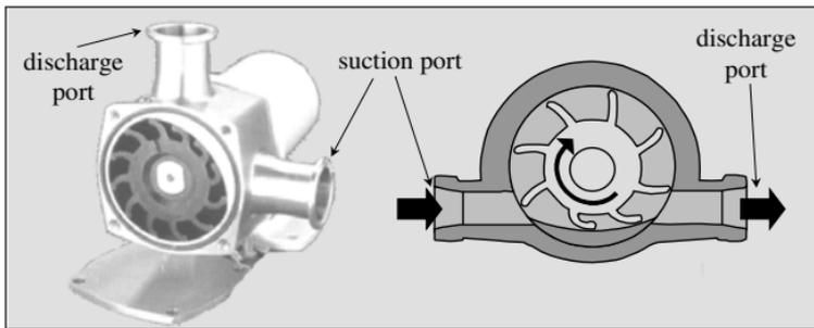
Figure 11-6 Flexible Impeller Pump
