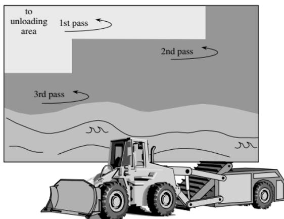
Figure 12-14 Elevating Scraper Treatment Pattern
