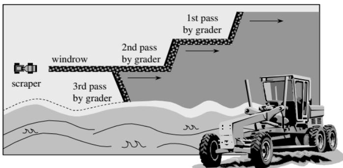
Figure 12-15 Motor Grader/Elevating Scraper Combination Treatment Pattern
