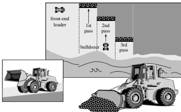
Figure 12-18 Bulldozer/Front-End Loader Combination Treatment Pattern
