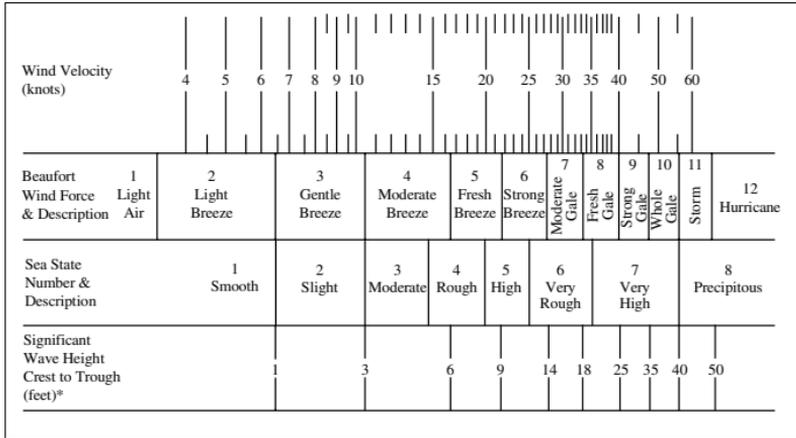
\*The average height of the highest 1/3 of the waves, assuming 1000 mile (1600 km) fetch, 25 hour duration, Bretschneider Spectrum
