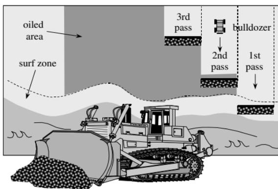
Figure 12-13 Bulldozer Treatment Pattern
