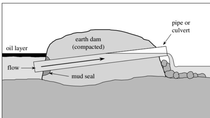
Figure 6-6 Inverted Weir
