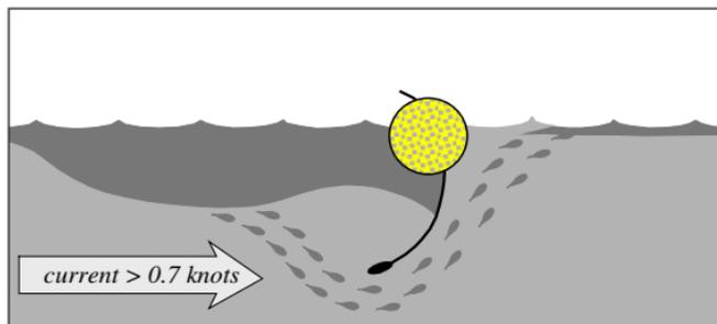
Figure 5-2 Entrainment Failure
