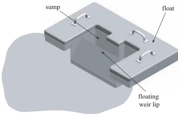
Figure 9-4 Self-Leveling Weir
