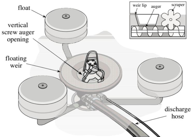
Figure 9-5 Weir with Integral Screw Auger
