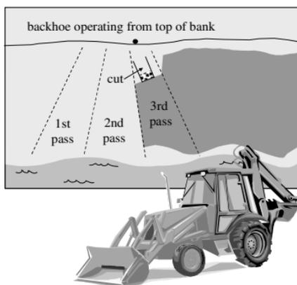
Figure 12-19 Backhoe with Front Bucket Treatment Pattern
