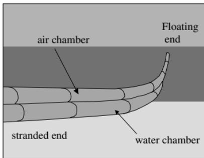
Figure 6-4 Shore-Sealing Boom
