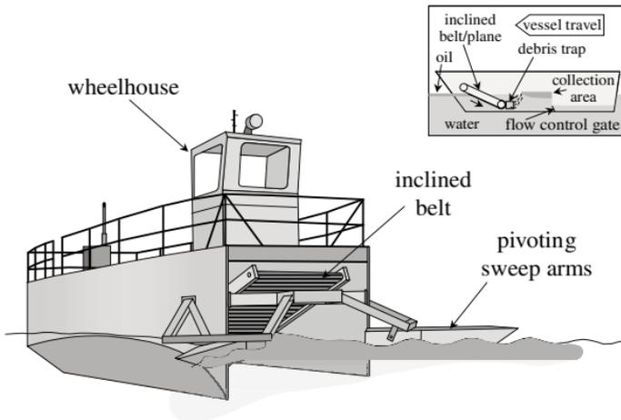
Figure 9-16 Submersion Plane/Belt Skimmer
