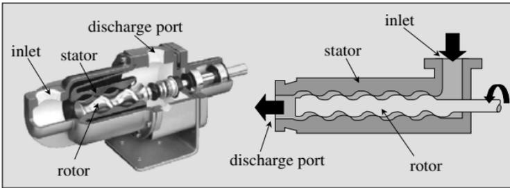
Figure 11-8 Progressive Cavity Pump
