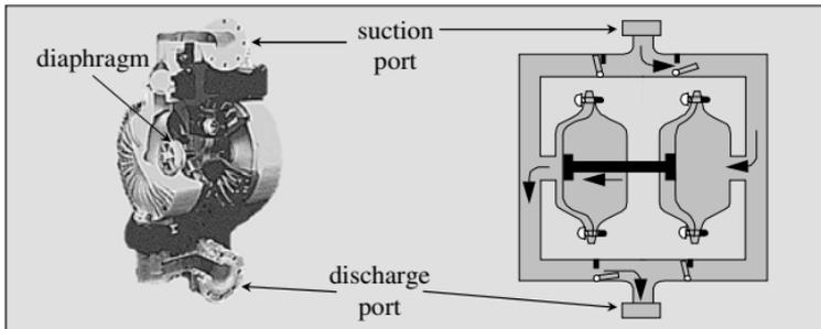
Figure 11-10 Diaphragm Pump
