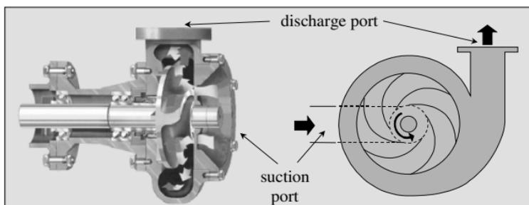
Figure 11-1 Centrifugal Pump
