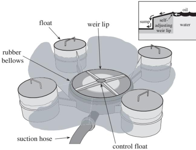
Figure 9-3 Self-Leveling Weir
