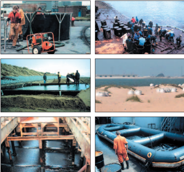
Examples of temporary storage on the shoreline and at sea (clockwise from top left): portable tanks; barrels; sacks; inflatable barges; in-built vessel tanks; lined pits.
