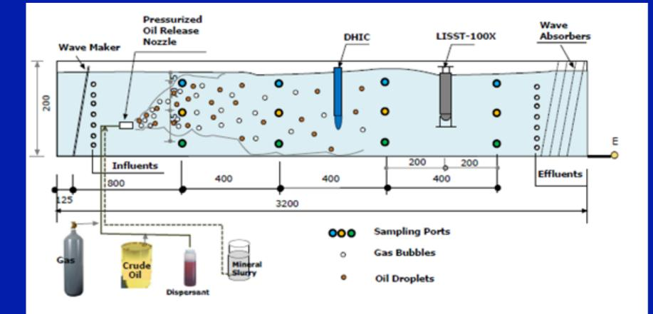
DHIC: Digital Holographic Imagery Camera, to measure particles  $20 - 2500 \ \mu m$ LISST: Laser in situ Scattering and Transmissometry, to measure particles  $2.5 - 500 \ \mu m$
