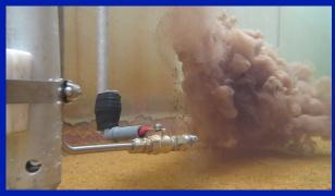
Oil Only Large droplets quickly rise to the surface
