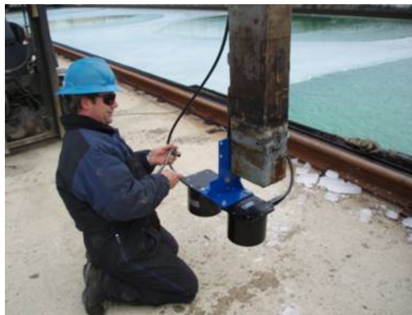
Figure 24. BioSonics DT-X Digital Scientific Echosounder sensor.
