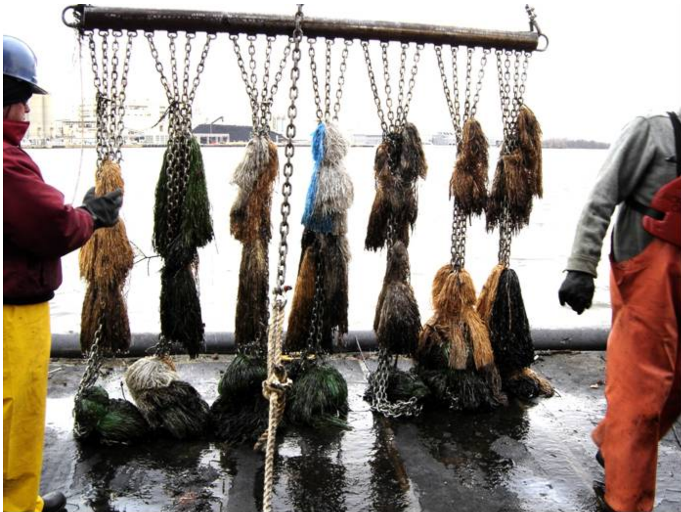
Figure E-2. The V-SORS used to search for and recover submerged oil.
