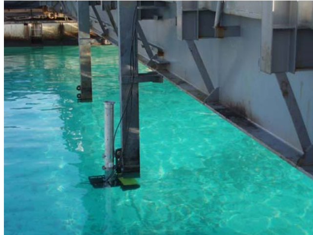
Figure 5. RESON 7125 SeaBat system mounted on the OHMSETT tank.
