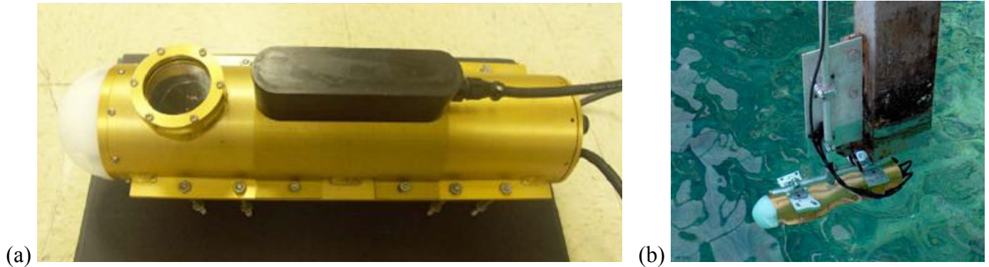
Figure 20. EIC FP probe (a) close-up and (b) in the test tank at OHMSETT.
