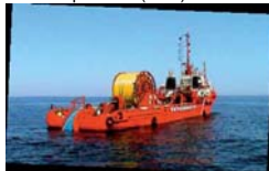
Cable laying ship
