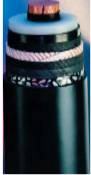
400-kV XLPE cable. The copper conductor is divided into five segments to reduce skin effect losses.
