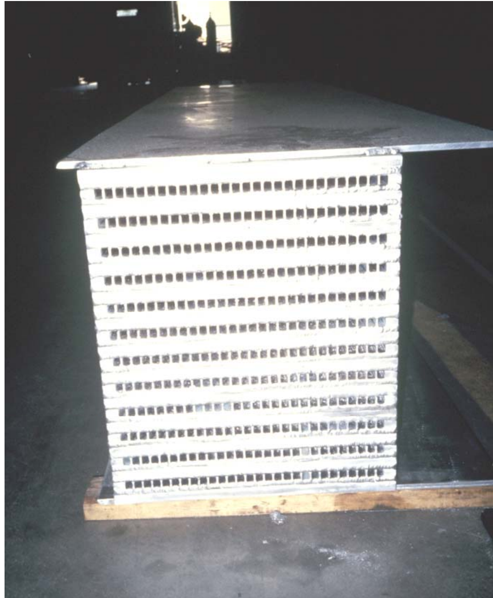
Surface Condenser: Extruded Water Channels
