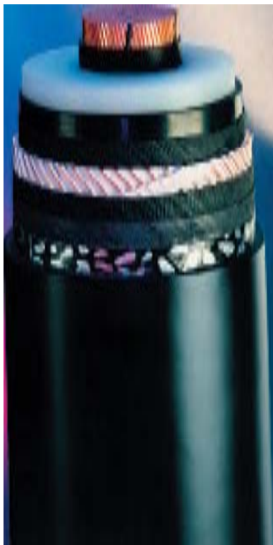
400-kV XLPE cable. The copper conductor is divided into five segments to reduce skin effect losses.
