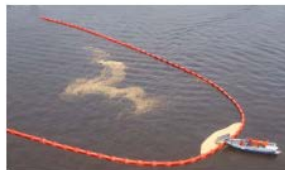
Mechanical Recovery: Booms & Skimmers
