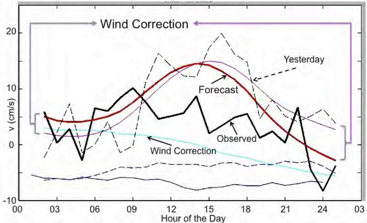
Figure 9. Sample surface current forecast results for 1 July 2006 for which a low-pass-filtered version of the observed north-south surface currents for the day prior have been persisted forward and corrected using the linear wind transfer function model applied to the difference between observed and forecast winds.
