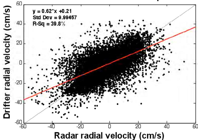
Figure 7. Combined drifter- versus HF radar-derived radial current comparisons for all radar sites for the NPS student cruise (upper) and CRRC drifter experiment (lower). The best-fit lines (red bold) are shown for each experiment along with the standard deviation about those lines.
