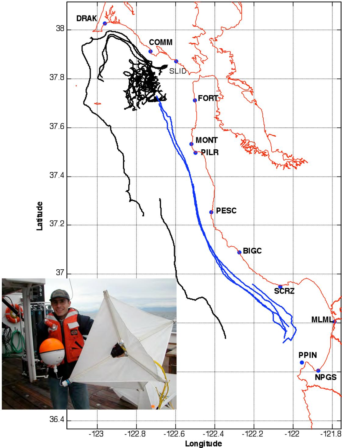
Figure 5. NPS thesis student Francisco Almeida holding a Pacific Gyre Microstar surface drifting buoy, including the electronics-housing surface float, tether, and tristar drogue element (inset), surface trajectories from the April CRRC (black) and January NPS student (blue) experiments, and the locations of shore-based HF radar sites (4-letter codes).
