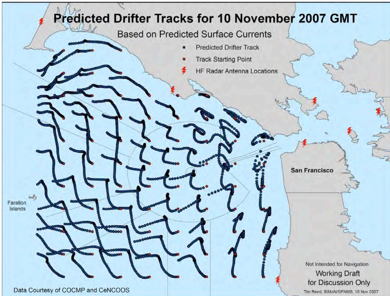
Figure B1. Example forecasted particle trajectories over a twenty four hour period from HF radar-derived surface currents plotted using a GIS program.
