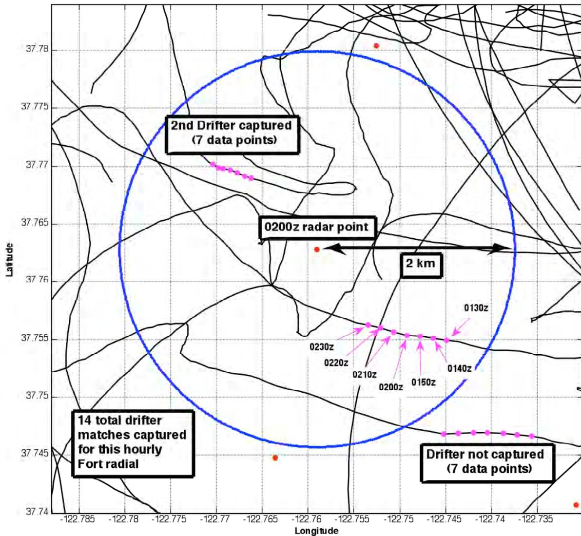
Figure 6. Example radar versus drifter data pairing. For each hourly radar grid point, such as the center symbol highlighted here for 0200Z, drifter data points corresponding to plus or minus 30 minutes and less than 2 km away from the center of the radar grid point were captured (magenta points inside blue circle for this example). This example has 14 total 10-minute velocity observations from drifter matches.
