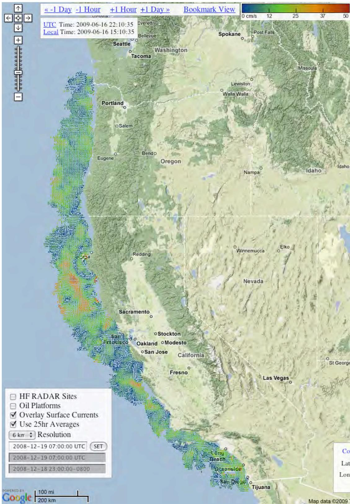
Figure 2. HF radar-derived surface current coverage along the U.S. west coast on the day COCMP operations were suspended (19 December 2009).
