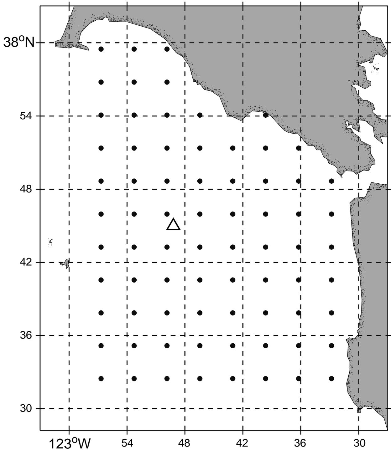
Figure 3. Region of the Gulf of the Farallones offshore San Francisco and the Golden Gate showing the initial locations (•) of surface particle trajectories computed from HF radar-derived currents together with the location NOAA/NDBC buoy 46026 (triangle).
