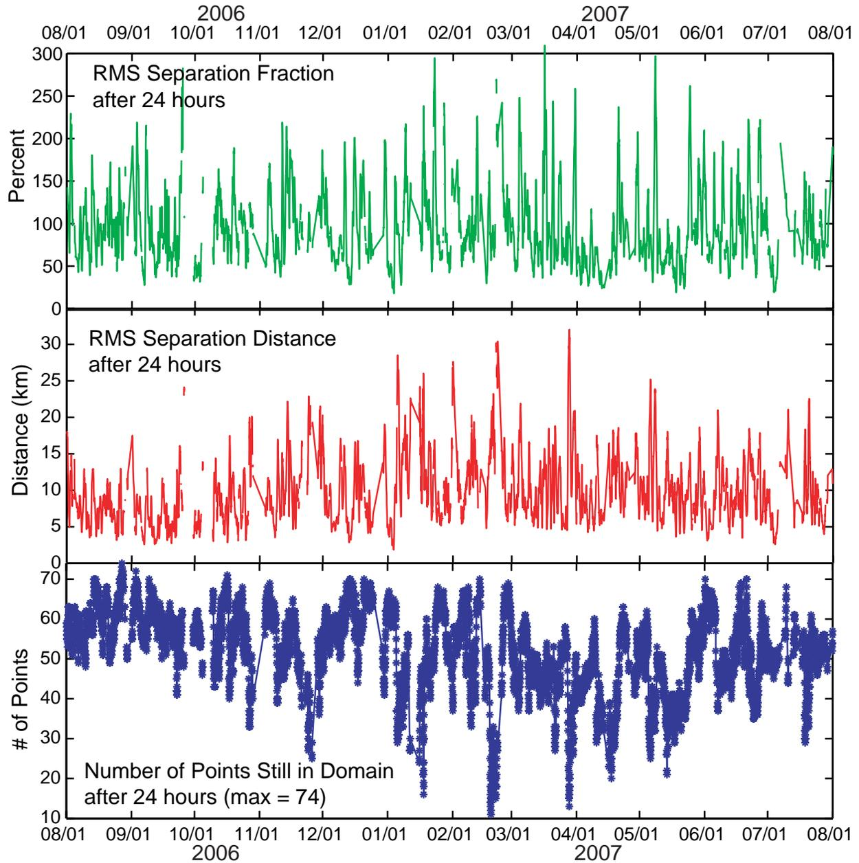
Figure 4. Hourly statistics of the RMS separation distance after 24 hours between the positions of forecasted and observed particle trajectories (middle) for the analysis grid in Figure 3. The fractional separation as a function of the RMS movement in the trajectories based on observed currents (upper) and the number of matching points remaining in the analysis domain after 24 hours (lower) are also shown.
