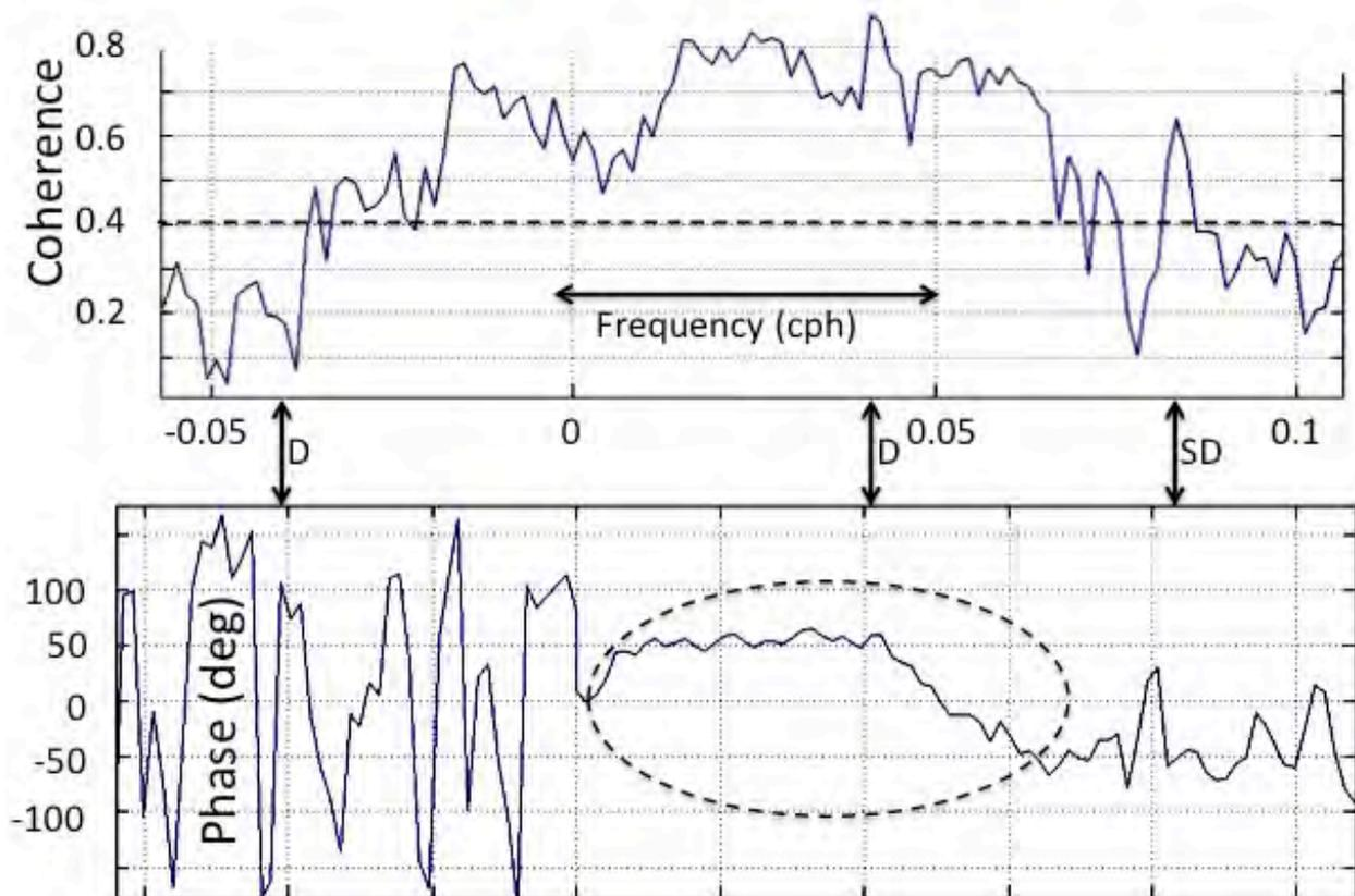
Figure 8. Coherence (upper) and phase (lower) between vector wind and HF radar-derived surface currents at the NDBC 46042 mooring location offshore Monterey Bay. The signals are coherent above the 95% confidence level (dashed line) over a broad frequency range from subtidal frequencies up to, approximately, diurnal frequencies. The phase offset in this band is consistently 50 degrees for the clockwise fluctuations with HF radar-derived surface current to the right of the wind forcing.
