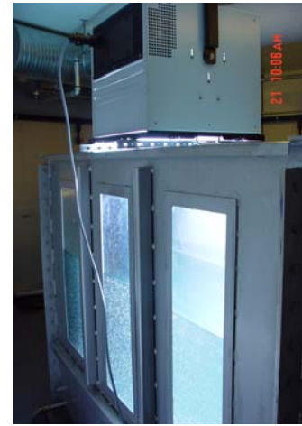
Figure 3.2 Meso-scale flume at SINTEF for long-term weathering studies of oils and petroleum products.
