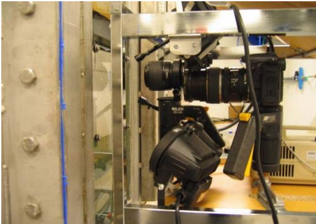
Figure 3.5. Picture of the still photo rig used in the experiments. In some tests, two cameras were used, one for capturing the full size of the screen, and one for close ups (macro lens). Lamps were mounted on the rig to give sufficient light conditions.
