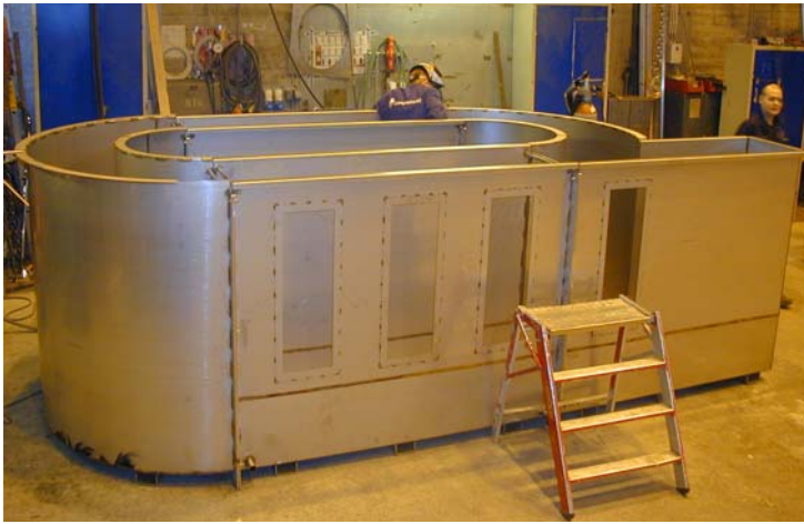
Figure 3.2 Meso-scale flume at SINTEF for long-term weathering studies of oils and petroleum products.
