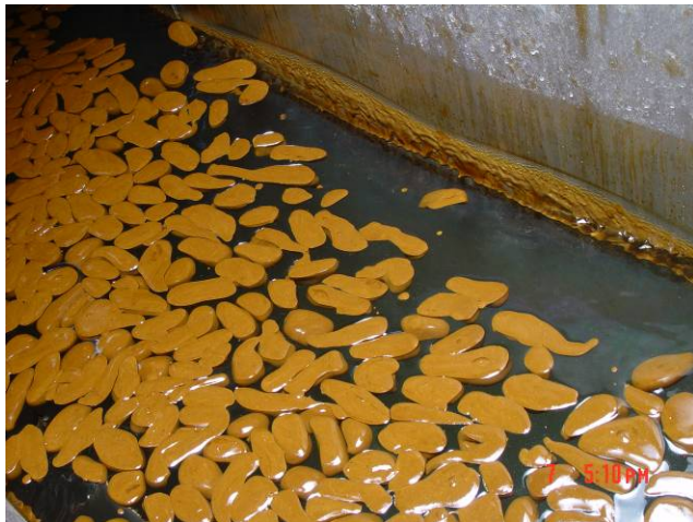
Figure 10.17 Images at various times in the flume experiment with Troll at 5°C and artificial sunlight.
