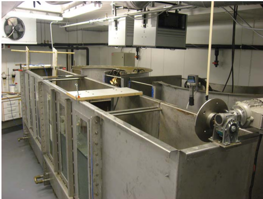
Figure 3.1. Sketch and photograph of the set-up for the breaking wave experiments. In the photograph, the semi-circular ends of the flume in its elliptical configuration can be seen to the right of the straight flume section in the foreground.
