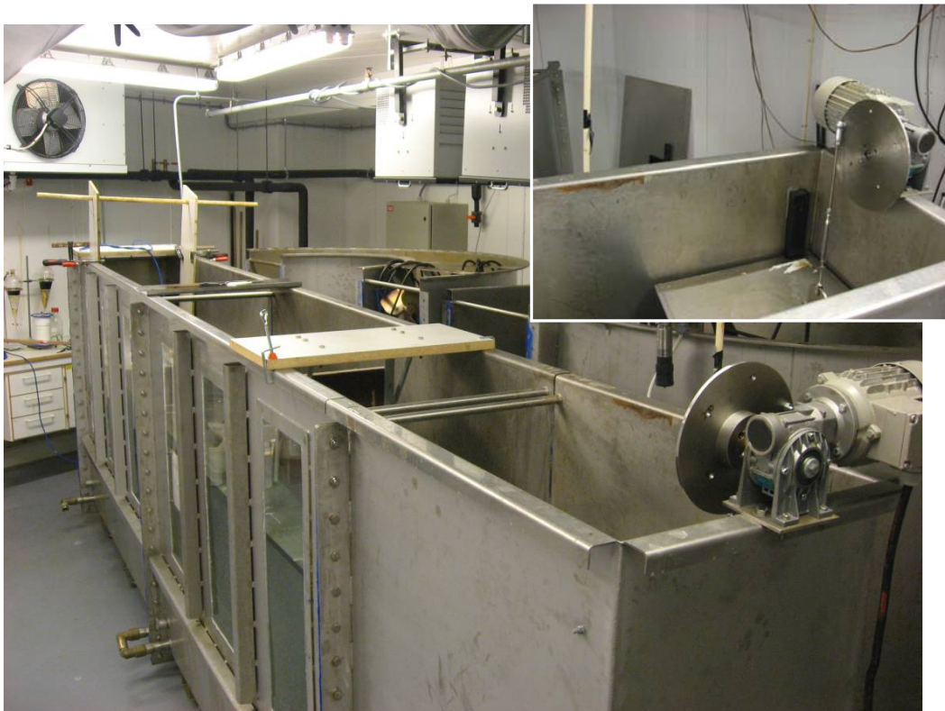
Figure 3.15. Picture of modified flume. Inserted: picture of wave generator.
