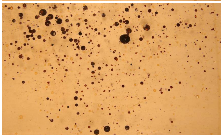
Figure 4.18. Examples of pictures from plunging jet experiments with Troll crude at 13°C. Pictures of droplet clouds obtained in three subsequent pictures 1 hour after start of the flume test. Picture numbers are given to the right of each picture. Note that the picture sequence is obtained within a time period of about 5 seconds.
