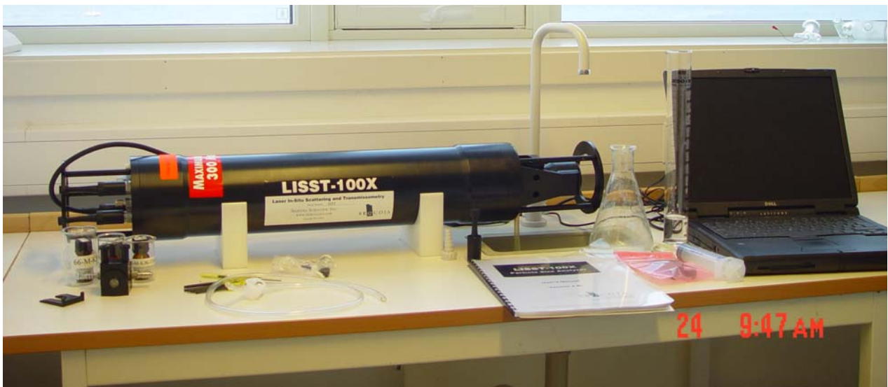
Figure 3.3 LISST-100x for measuring droplet sizes in the meso-scale flume. The instrument can be placed in situ or be used bench-top with a flow-through pump system.
