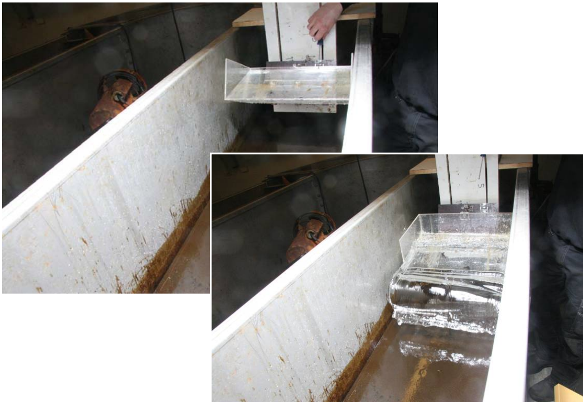
Figure 3.7. Close up of plunging jet arrangement. The water filled Plexiglas tray produces a plunging water jet when tilted to a horizontal position. The free fall height is adjusted by moving the container up or down in slides cut into the fastening board.
