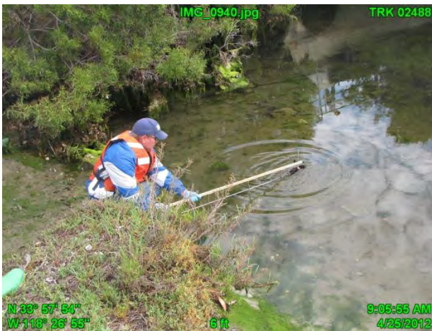
Photograph 23 Ballona Wetlands sample gathering. Personal flotation device (PFD) must be worn. Important: Keep personnel and 'footprint' to a minimum in the Wetlands.
