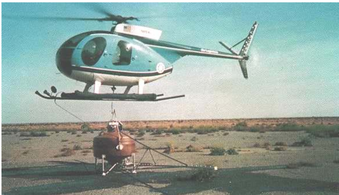
Figure 15.8 Helicopter "Slung Bucket" Spray System
