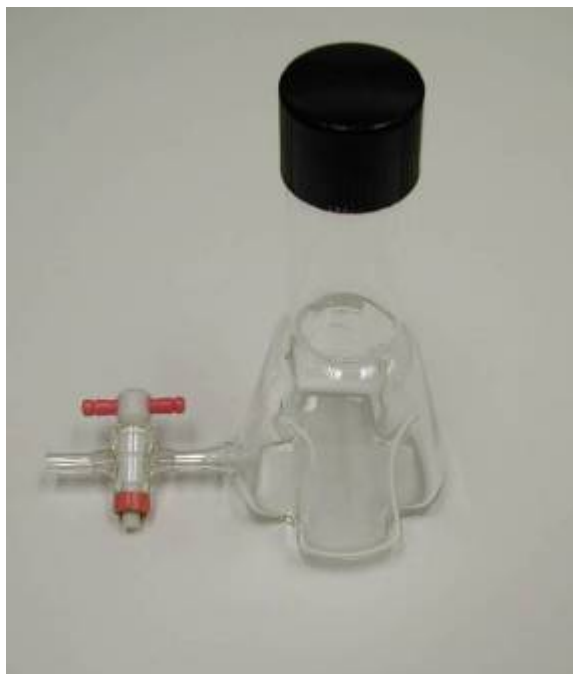
Figure 7.5 US Swirling Flask Modified to Provide Higher Energy and Improve Reproducibility
