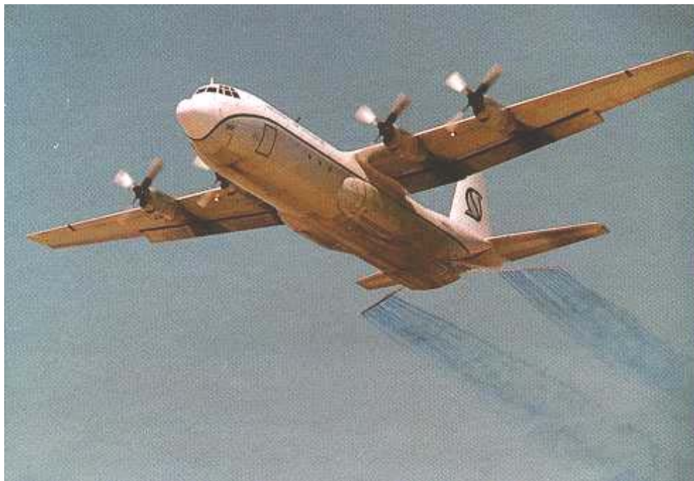
Figure 15.5 Aerial Application of Corexit 9527 (Dyed Blue) from Southern Air L-100 Using ADDS PACK System in Alpine, Texas Test (Courtesy of Shell)
