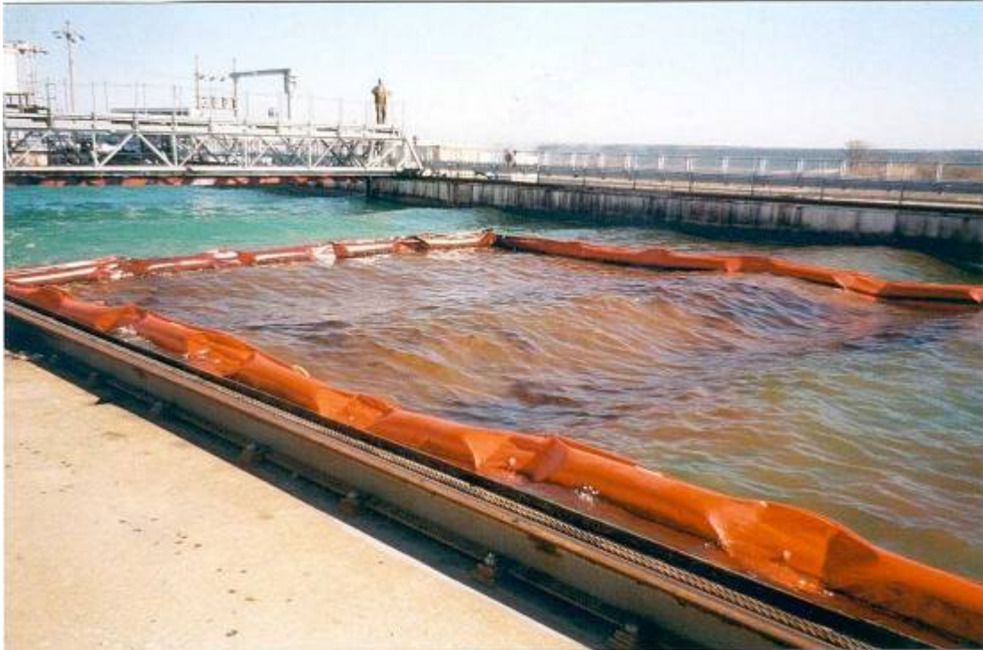
Figure 7.7 Dispersant Test on ANS Crude at OHMSETT
