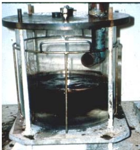
Figure 7.3 Mackay, Nadeau, Steelman (MNS) Test. Energy Provided by Air Stream (Highest Energy)
