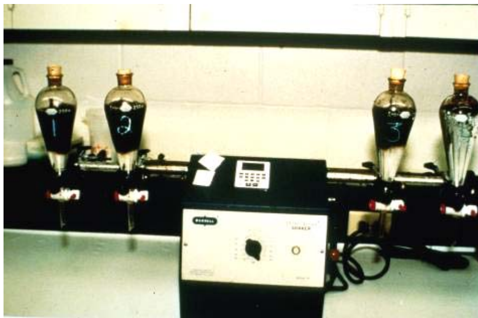
Figure 7.6 EXDET Test Used by ExxonMobil. Energy Supplied by Rocking (Medium Energy)
