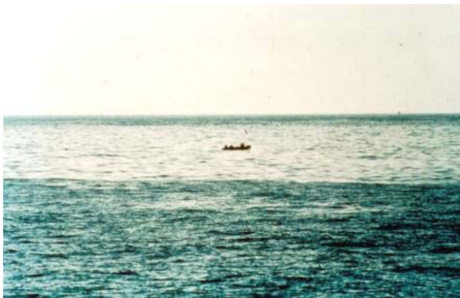
Figure 8.5 Slicks in the 1997 North Sea Trials Were Extensive. Oil is in the Bright Area.
