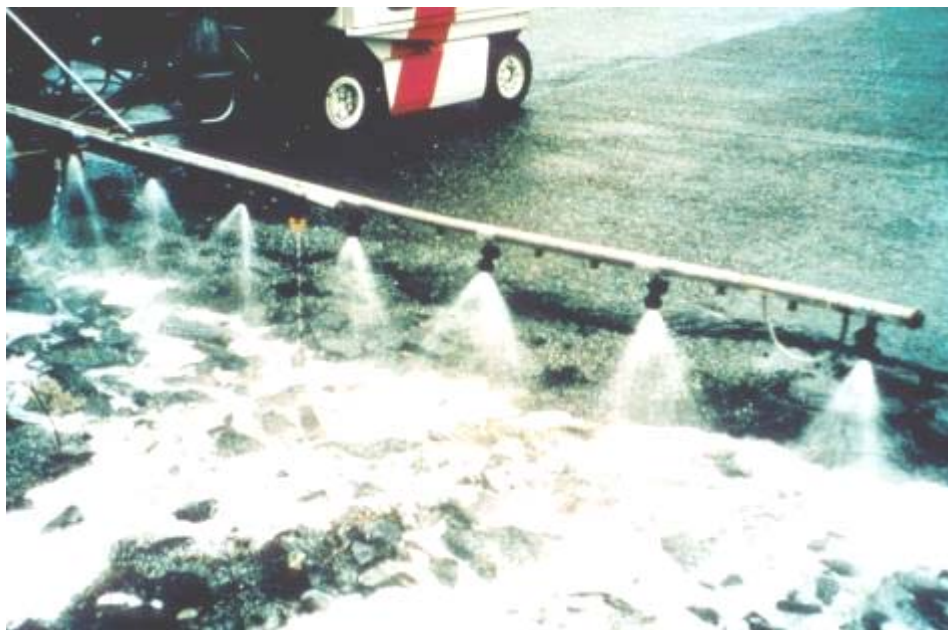
Figure 15.12 Uneven Spray Distribution During Test
