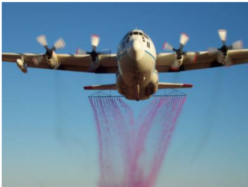
Figure 15.3 Aerial Application of Chemical Dispersants from MSRC's C-130A, Supplied by International Air Response, Inc. (courtesy of MSRC)
