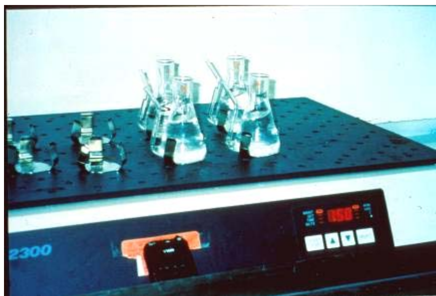
Figure 7.3 Mackay, Nadeau, Steelman (MNS) Test. Energy Provided by Air Stream (Highest Energy)
