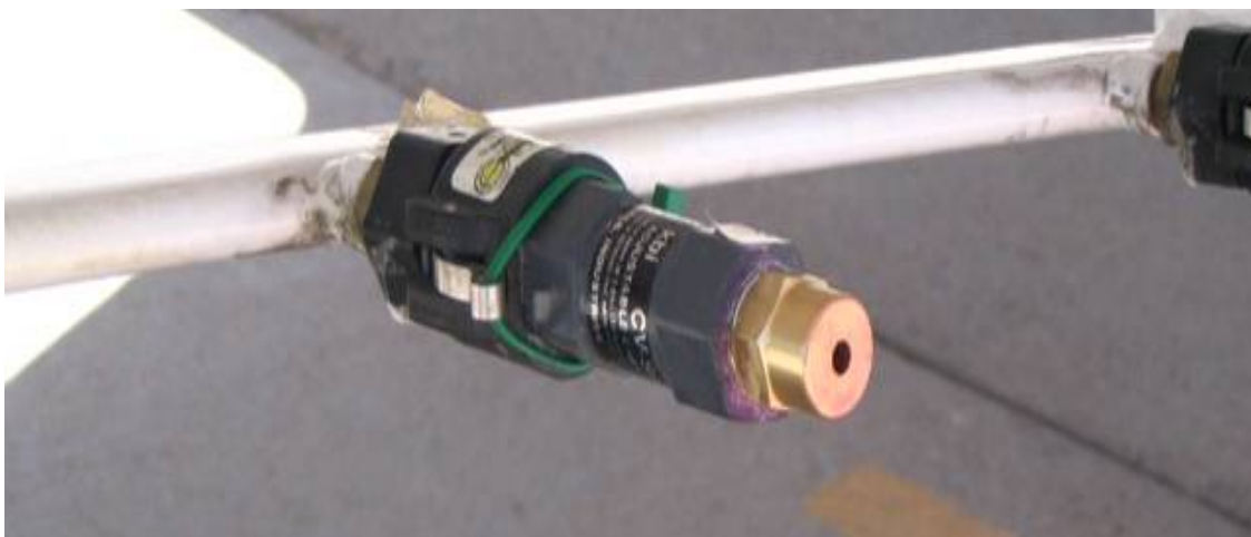
Figure 15.6 Close-Up View of Spray Boom Nozzle (BETE NF 70) (Courtesy of MSRC)
