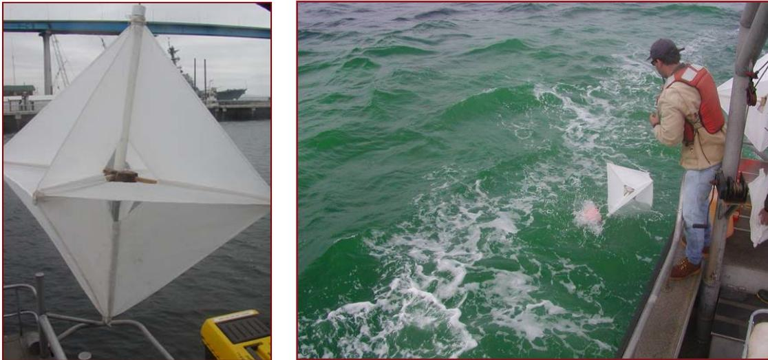
**Figure 3-4. Drogue (kite) tied with a 1-, 2-, 4-, or 5-m tether to the drifter floats/transponders (left) and release of a drogued drifter/transponder into the dye plume from the MSRC *Response 2* on 8 November 2005 (right).**
