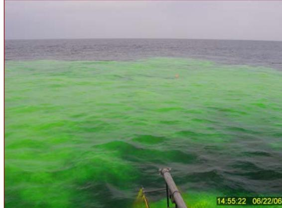
**Figure 3-2. Fluorescein dye release from the spray booms on the starboard side of the MSRC *Response 2* (left) and the appearance of the dye mixing into the water surface six minutes after release on 22 June 2006 (right).**
