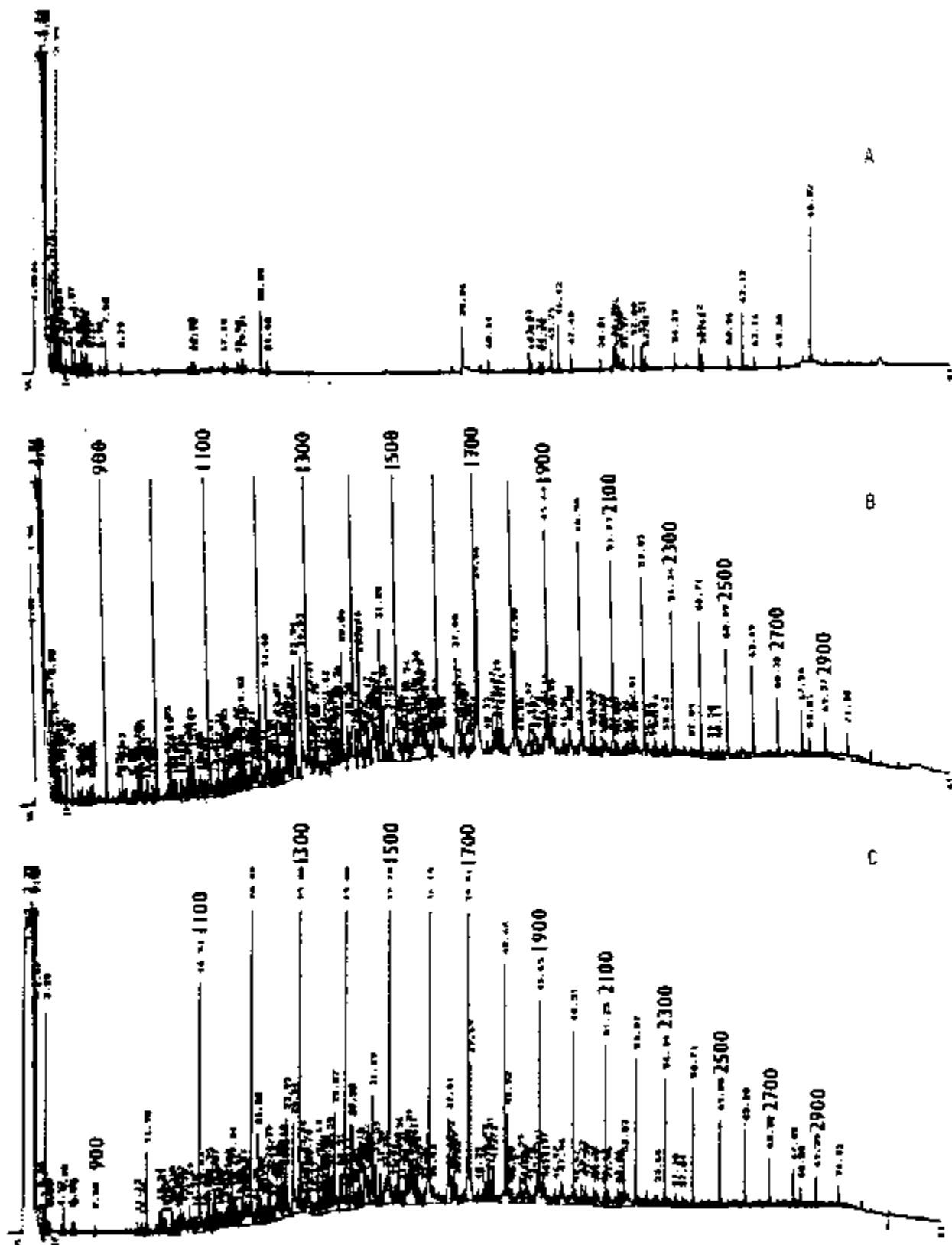
FIGURE 6-27. FID-GC chromatograms of filter extracts from Wave Tank #3 showing Dispersed/Particle Bound oil at: (A) Prespill Blank, (B) 1 hour, and (C) 8 hours after a spill of 16 liters of Prudhoe Bay crude oil.
