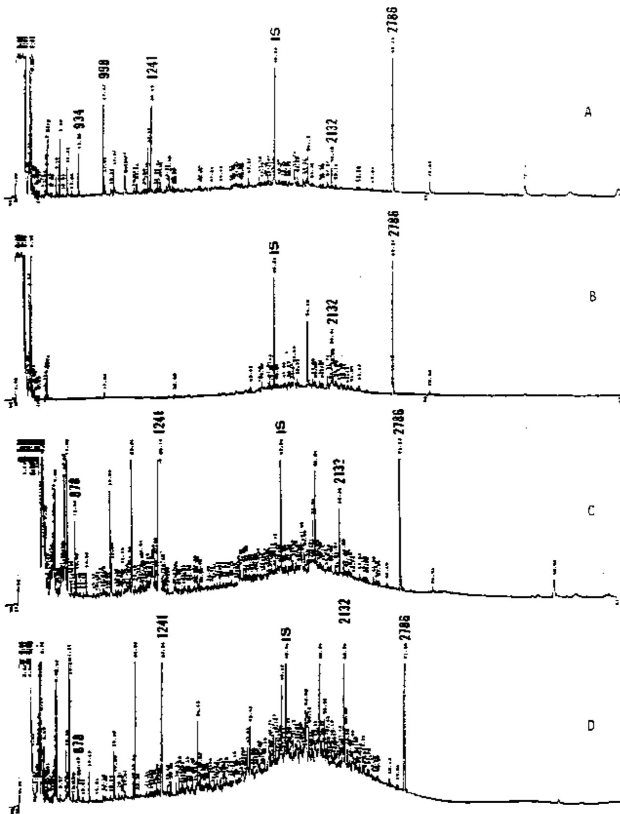
FIGURE 7-18. FID-GC Chromatograms of the Polar Seawater extract fractions from the SIO Summer 1981 continuous-flow weathering study: (A) and (B) two experimental tanks at day 9; (C) and (D) at day 23 post-spill time. (IS= Internal Standard).
