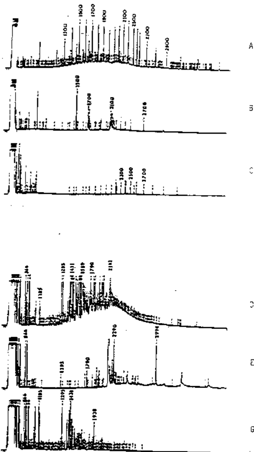
FIGURE 6-17. FLAME IONIZATION DETECTOR CAPILLARY GAS CHROMATOGRAMS FROM KB-3 (KASITSNA BAY COMPOSITE SEDIMENT) OIL/SPM INTERACTION STUDIES: (A) ALIPHATIC HYDROCARBONS IN THE OIL EXPOSED SEDIMENTS; (B) BACKGROUND LEVEL ALIPHATIC HYDROCARBONS MEASURED IN UNEXPOSED SEDIMENT; (C) ALIPHATIC HYDROCARBONS IN THE WATER COLUMN EXTRACT; (D) AROMATIC HYDROCARBONS IN THE OIL EXPOSED SEDIMENTS; (E) BACKGROUND LEVEL AROMATIC HYDROCARBON COMPONENTS MEASURED IN THE UNEXPOSED SAMPLE; AND (G) AROMATIC HYDROCARBONS IN THE WATER COLUMN EXTRACT.
