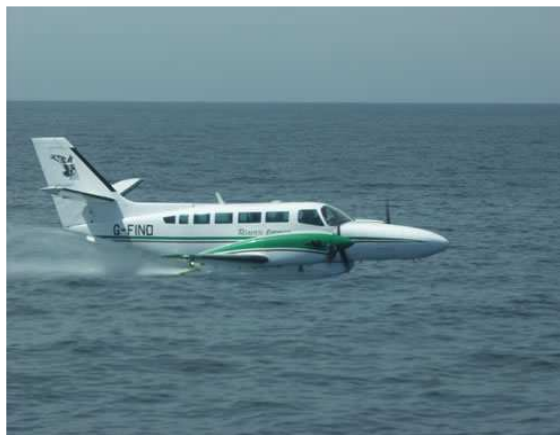
Cessna from OSRL equipped with a spraying POD applying dispersant during Depol 04 sea trial [Cedre]
