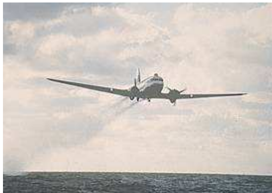
Aerial application of dispersant by a DC3 during the Sea Empress incident [MPCU]
