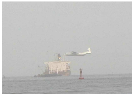
Dispersant spraying operation with the C130 Hercules during the Tasman Spirit incident in Pakistan- [picture from http://www.spillcon.com/2004/papers/O'BRIEN.pdf ]
