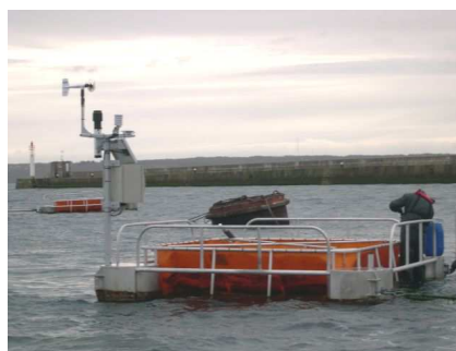
Experiment in floating cells equipped with meteorological monitoring [Cedre]
