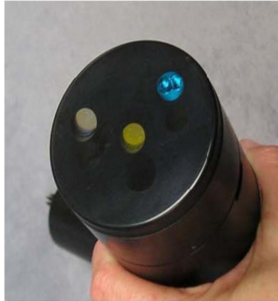
**Figure 22: Wet Labs Environmental Characterization Optics (ECO) triplet sensor.**
