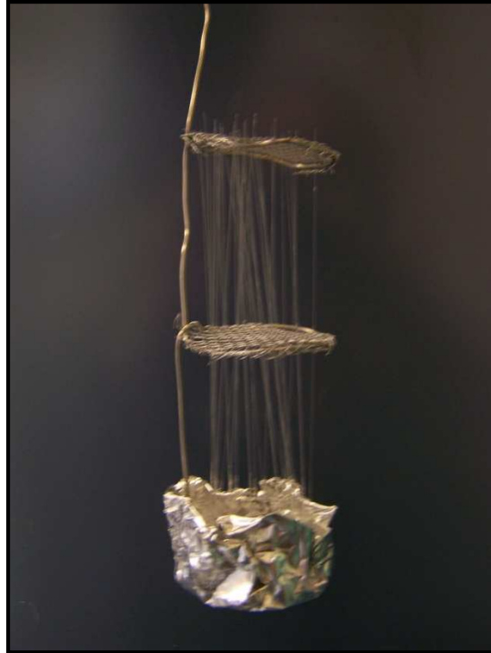
Figure 1. Metal rack constructed from stainless steel wire and screening to assist SPMEs to reach equilibration with PRCs.
