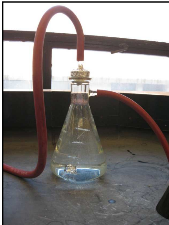
Figure 2. Laboratory set up to verify SPME loss rate incorporating an Erlenmeyer flask attached to a laboratory faucet to simulate turbulent conditions in the field.
