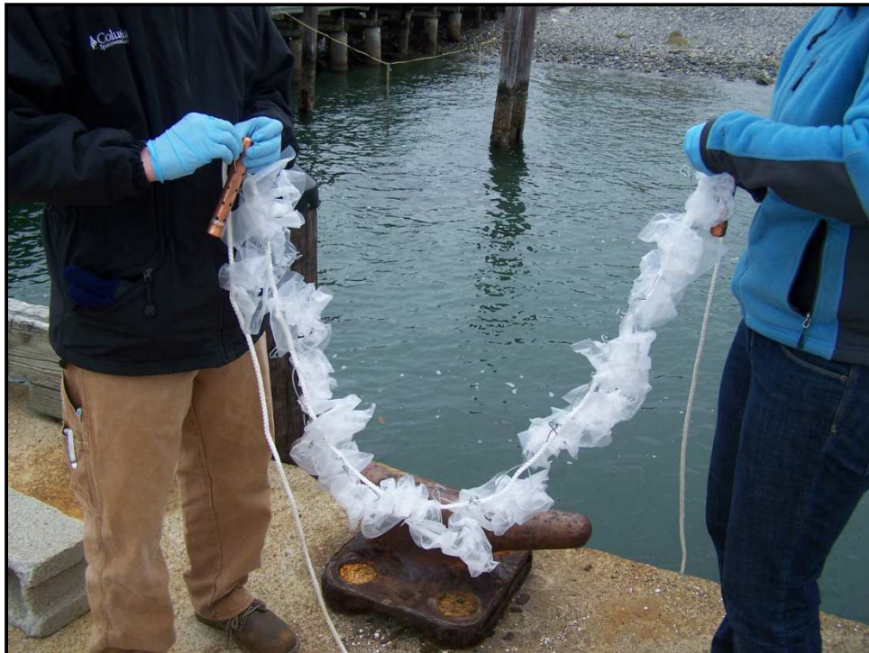
Figure 4. PEs threaded on stainless steel wire (A) and attached to deployment line (B) for the field deployment in Narragansett Bay.
