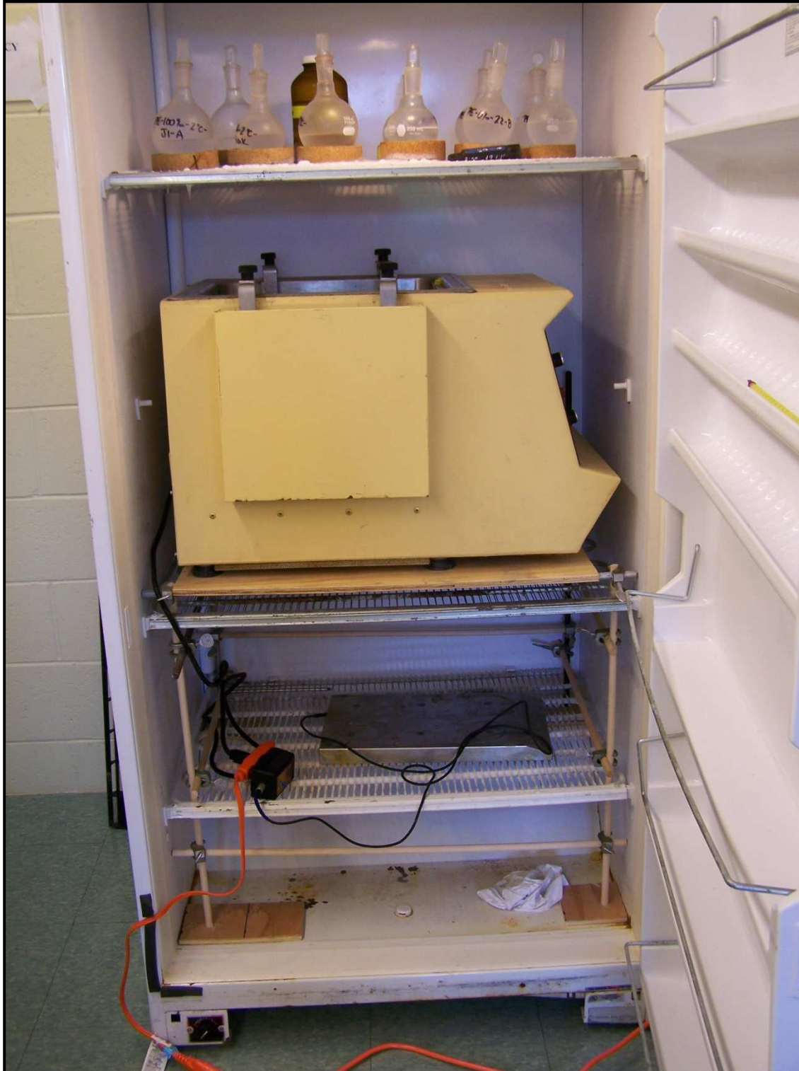
Figure 3. Freezer arrangement incorporating a shaker table to hold the SPME samples and a stir plate for the PE samples to complete the -15\text{ }^{\circ}\text{C} experiment.
