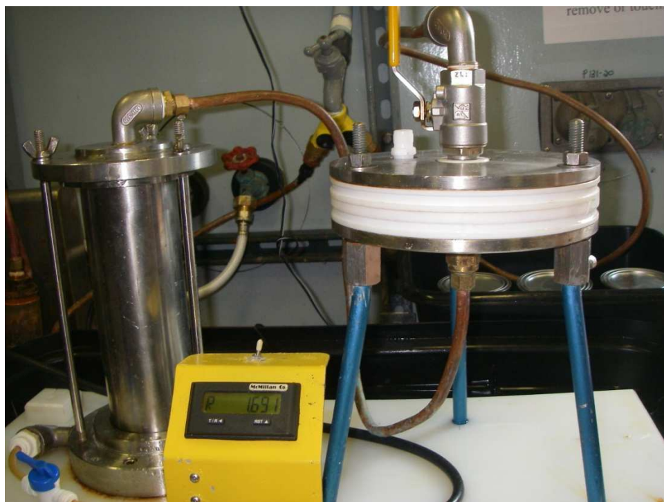
Figure 6. Active sampling arrangement with PUFs inserted in the tall cylinder (left) and filters placed in the flat platform (right) to collect dissolved PAH concentrations present in Narragansett Bay.
