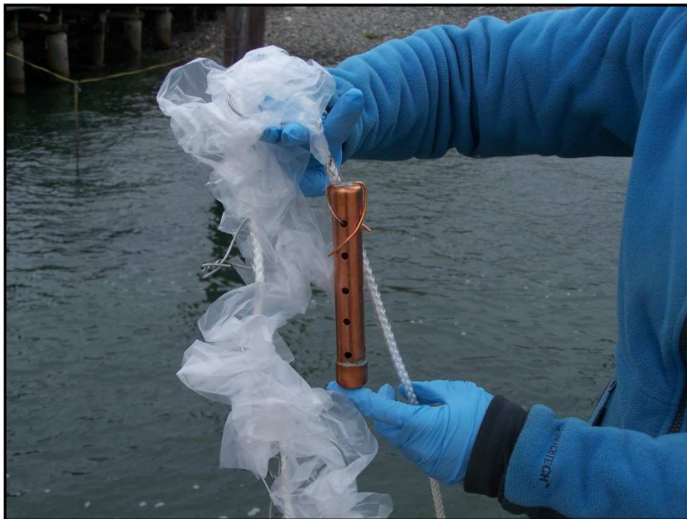
Figure 5. Copper housing manufactured to house SPMEs during the field deployment (A) and copper housing attached to deployment line with stainless steel wire for the field deployment in Narragansett Bay.
