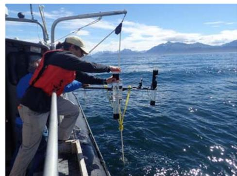
UNH graduate student Jesse Ross deploys particle traps in the water column this August. Jesse deployed 14 traps through the course of the summer. Each trap remained in the water column for one and a half hours before being retrieved.
