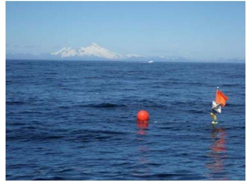
Tracking buoy and flag mark the site for recovery. Once retrieved, the samples that settle to the bottom will be collected and transported to New Hampshire for the laboratory experiments.
