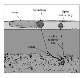
Figure 5-16 Boom Anchoring Assembly
