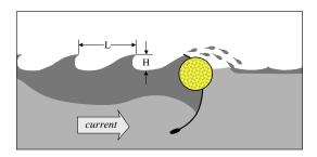
Figure 5-4 Splashover Failure
