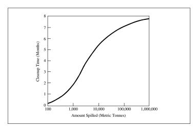
Figure 1-6 Spill Size Versus Duration of Cleanup
