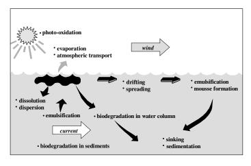
Figure 4-1 Processes Acting on Spilled Oil
