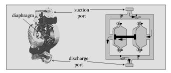
Figure 11-10 Diaphragm Pump
