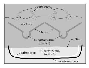
Figure 12-6 Low Pressure Flushing
