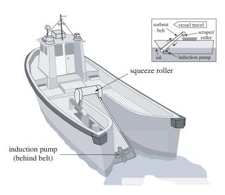
Figure 9-13 Sorbent Lifting Belt
