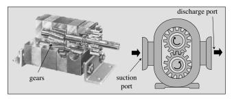
Figure 11-3 Gear Pump
