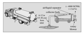
Figure 11-13 Air Conveyor
