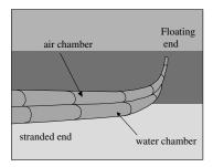
Figure 6-4 Shore-Sealing Boom
