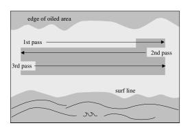
Figure 12-11 Tractor/Ripper Treatment Pattern
