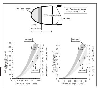
Figure 8-1 Estimating Boom Holding Capacity
