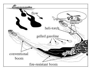
Figure 8-3 Typical In-Situ Burning Operation
