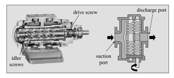
Figure 11-4 Intermeshing Screw Pump
