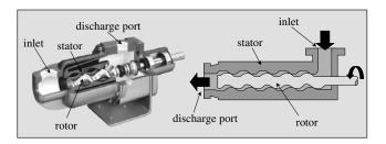
Figure 11-8 Progressive Cavity Pump
