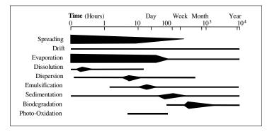
Figure 1-11 Processes Versus Time Elapsed Since the Spill
