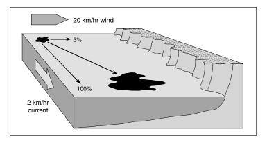
Figure 4-2 Movement of Oil on Water
