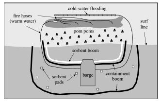
Figure 12-7 Low-Pressure, Warm-Water Washing/Cold-Water Flooding
