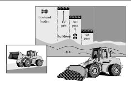
Figure 12-18 Bulldozer/Front-End Loader Combination Treatment Pattern
