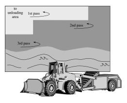
Figure 12-14 Elevating Scraper Treatment Pattern
