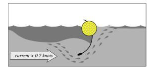
Figure 5-2 Entrainment Failure
