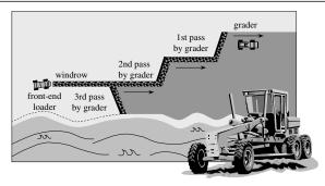
Figure 12-17 Motor Grader/Front-End Loader Combination Treatment Pattern
