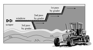
Figure 12-15 Motor Grader/Elevating Scraper Combination Treatment Pattern
