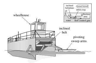
Figure 9-16 Submersion Plane/Belt Skimmer
