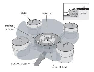
Figure 9-3 Self-Leveling Weir
