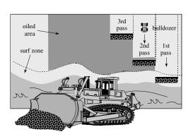
Figure 12-13 Bulldozer Treatment Pattern
