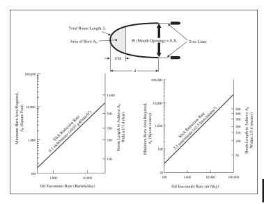
Figure 8-2 Estimating Area Required for Various Oil Encounter Rates
