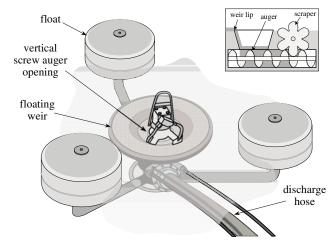
Figure 9-5 Weir with Integral Screw Auger
