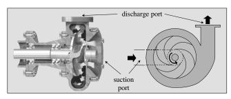
Figure 11-1 Centrifugal Pump
