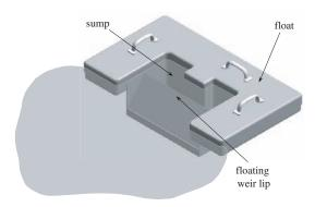
Figure 9-4 Self-Leveling Weir
