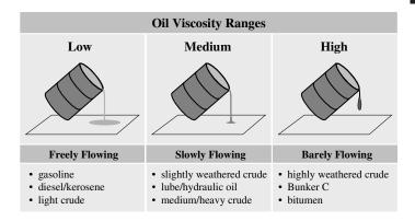
Figure 9-1 Oil Viscosity Ranges
