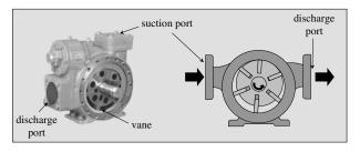
Figure 11-5 Vane Pump
