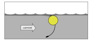
Figure 5-5 Submergence Failure
