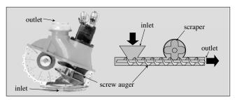
Figure 11-7 Screw/Auger Pump
