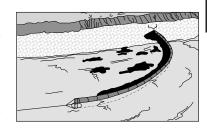
Figure 5-14 Shore-Sealing Boom
