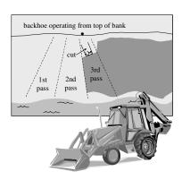
Figure 12-19 Backhoe with Front Bucket Treatment Pattern
