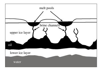
Figure 15-1 Melt Pools and Encapsulated Oil (From EPPR 1998)
