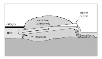
Figure 6-6 Inverted Weir
